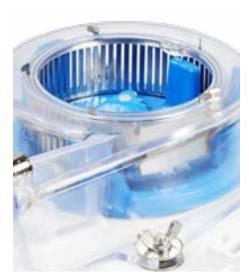
All Blade Retention Tabs (six) must, at all times, be twisted to secure the Blade and Blade Housing together or the Blade may shear off destroying the Blade Housing.
