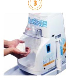
Put hands up to the machine to catch the clog. Tap foot pedal slightly and clogged ice will shoot out.
